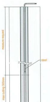
Cutting procedures only in the lower part. The cut can be done with blade for wood or aluminium.
